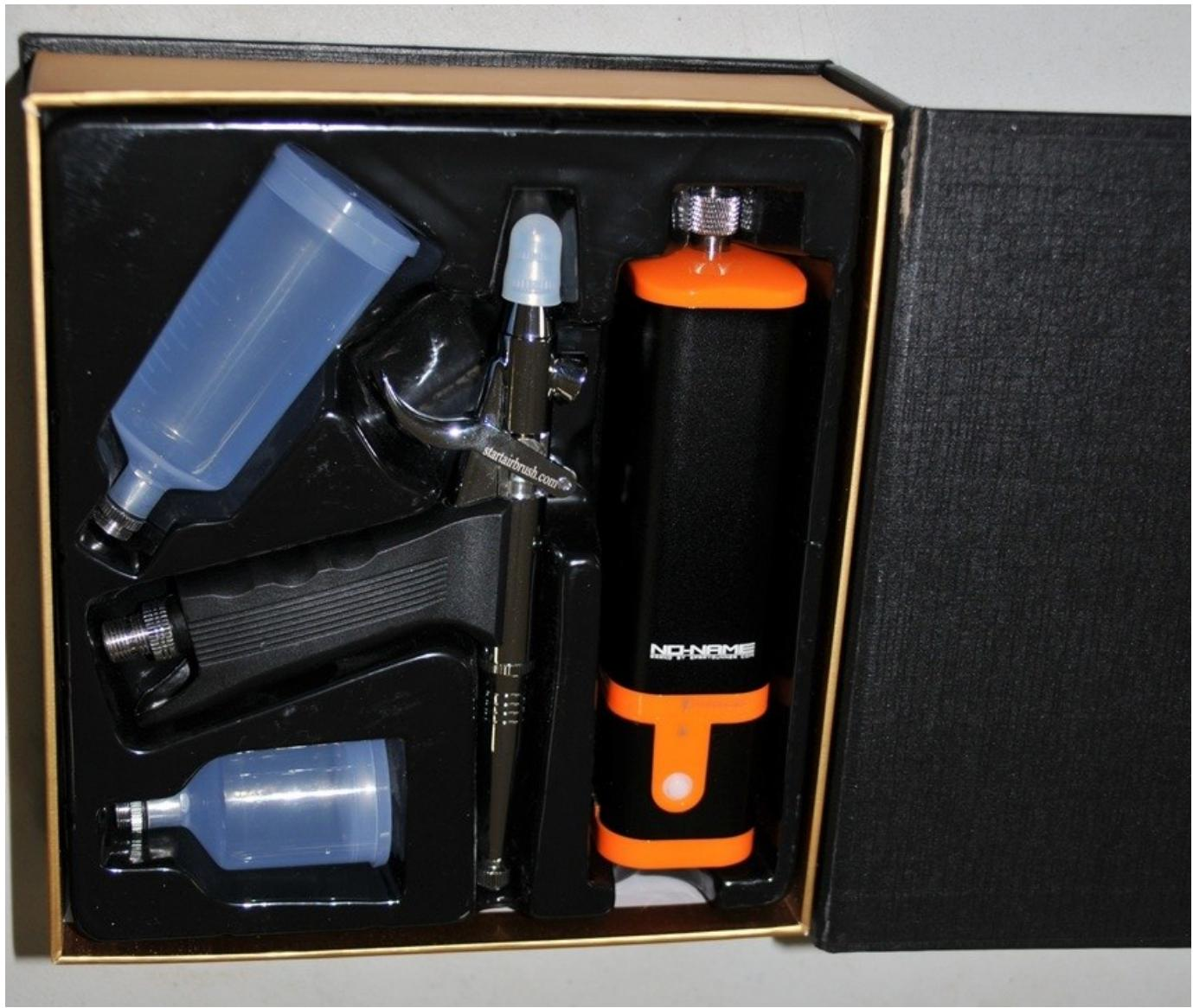
While at the 2025 International Plastic Modelers Society (IPMS) National Convention, Toni Levine discovered this portable airbrush with cordless micro-compressor. Known as the "No-Name", the unit is battery powered, and can be recharged via USB.2 batteries. It allows you to adjust air pressure for full control over your painting.
